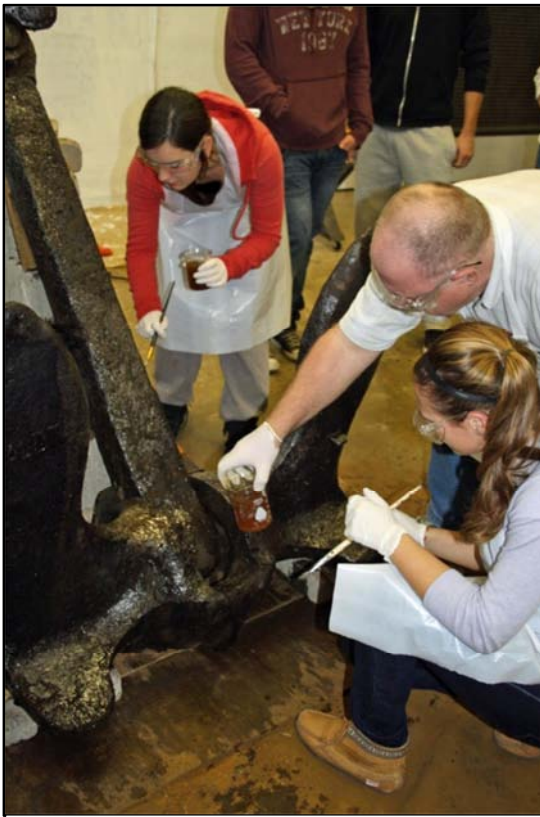
Tom Stretton's senior chemistry class applying tannic acid to the anchor. This process was directed by the Canadian Conservation Institute as the best way to preserve an iron artefact. (TISS)
